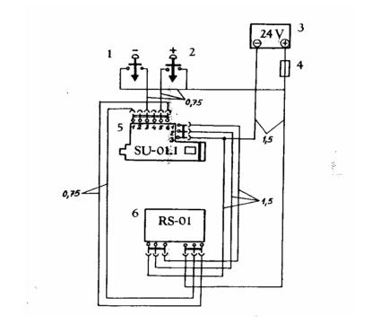
Fig. 1a - Electrical connexion of the airscrew unit
